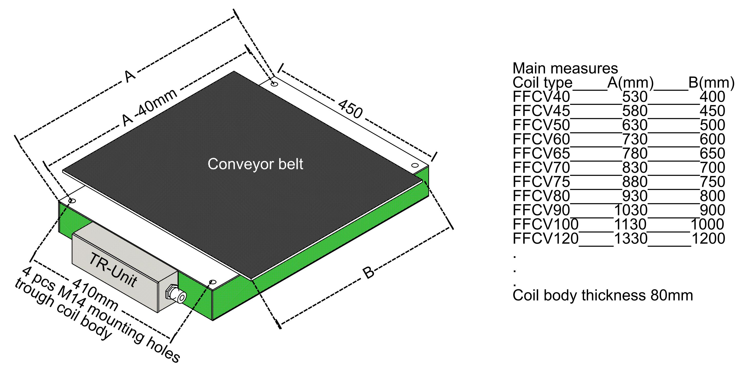
FFCV-coils especially for vibratory conveyors FFCV-coils have been protected against the influence of metallic constructions both under and the sides of the coil by a rigid alumunium body. The sensitive coils have been located very close to the upper surface under a glass fibre sheet.
